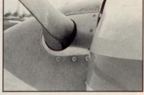
The modified Bonanza has four vernier controls that all look alike: The bottom right control opens and closes RamAire door. Other modifications include: turned back exhaust stacks (they used to extend outward at 45 degree angles); spinner seals around the propeller; and a fiberglass tailcone to reduce "intersection drag" between the elevators and the original tailcone.
